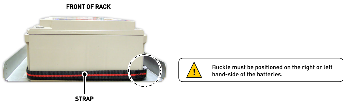
Figure 12 Securing the batteries (front of rack)
